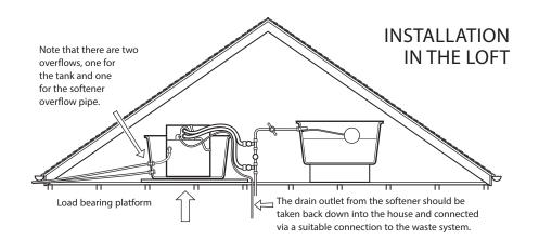
The Block Salt Softener may be installed in the loft or roof cavity but it should be within a safety tank. A suitable tank is a plastic roof storage tank sufficiently large to accommodate the block salt softener. Please note that it should be mounted on a board strong enough to spread the weight over a load bearing wall.
