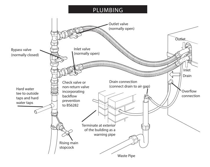
The diagram above shows how easy it is to install the Block Salt water softener. There are just four connections: mains water inlet, outlet, drain and overflow.
