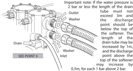
tube must not exceed 3m and the discharge point should be below the top of the softener. The length of the drain tube may be increased by 1m, and the discharge point above the top of the softener increase
